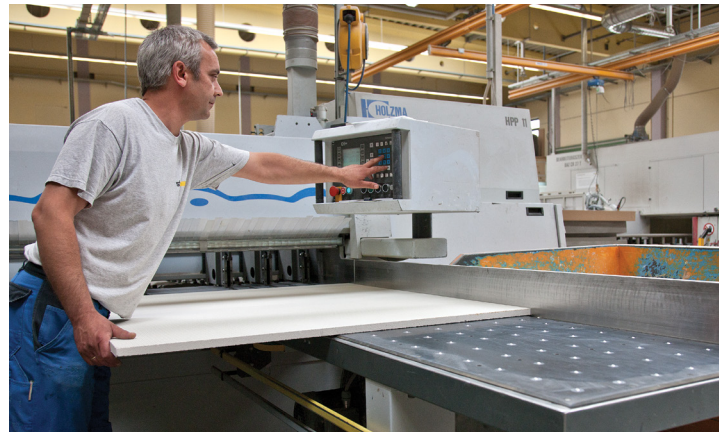
To the millimetre: StoVentec Glass panels are cut to their individual format
